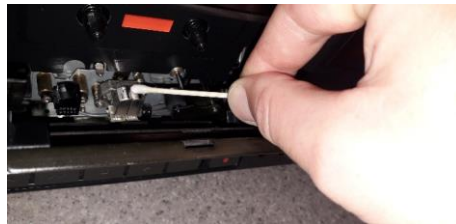
Image of how to clean a tape deck playback head with cotton bud.
