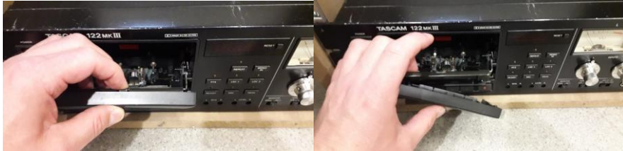
Image of how to slide the door off the Tascam
