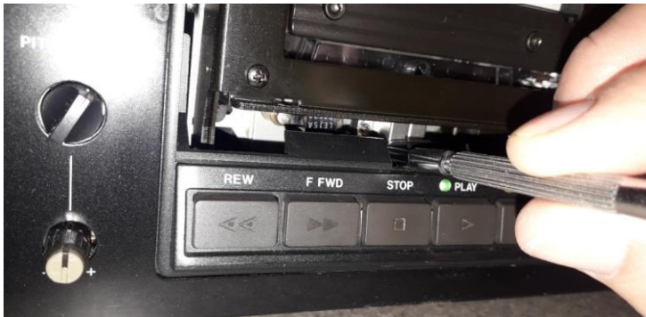
Image of using a small Philips screwdriver to manually adjust the azimuth
