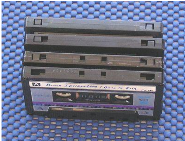
TOP to BOTTOM: FROM Type 1 Normal, Type 2 Chrome & bottom two Type 4 (one with the safety tabs removed).
