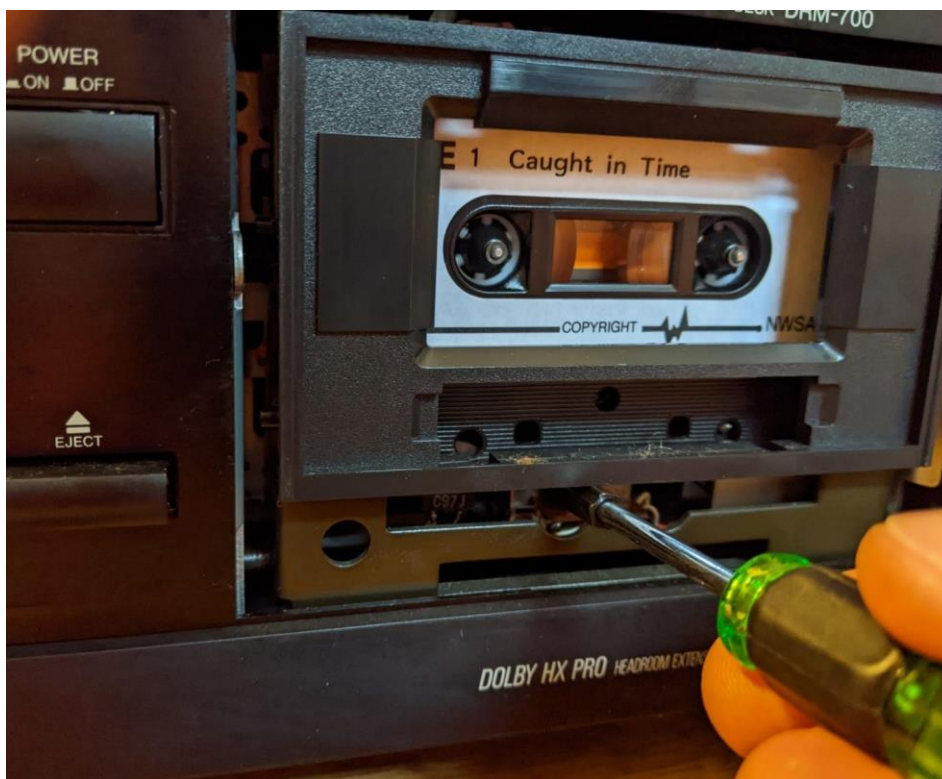
Image of using a 4mm hex driver to manually adjust the azimuth
