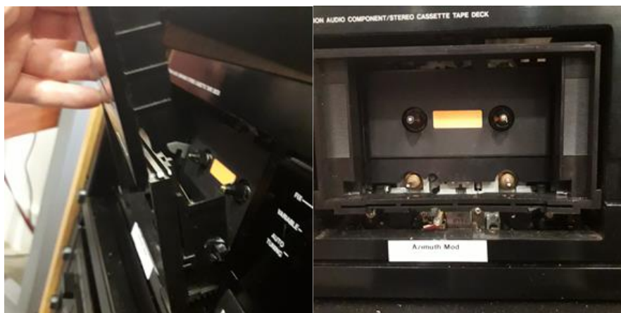
Image of how to slide the door off the Denon Deck
