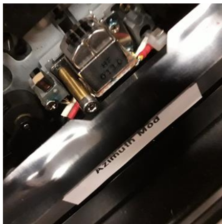
Image of Denon 790-R tape deck play head (marked HF0101 on its side)
